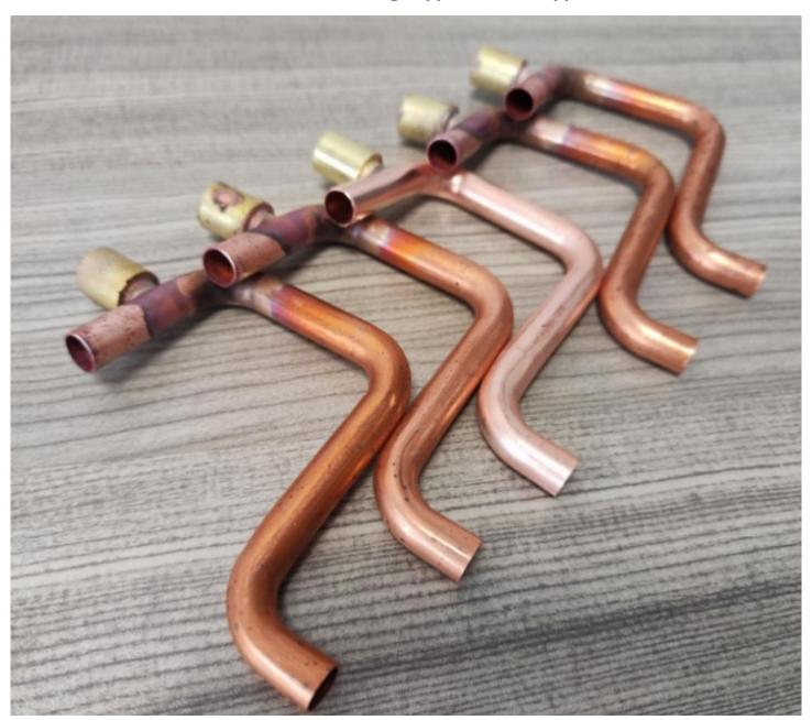
**Zhengzhou, Henan Apr 10, 2023 (**<u>Issuewire.com</u>) - FOCO Induction, a renowned Chinese induction heating machine manufacturer, has recently showcased its groundbreaking induction brazing copper to brass application, utilizing a 10 kW handheld induction brazing machine. The advanced technology is designed to provide rapid, precise, and efficient brazing, making it ideal for precision parts in industries such as HVAC, plumbing, and automotive.
